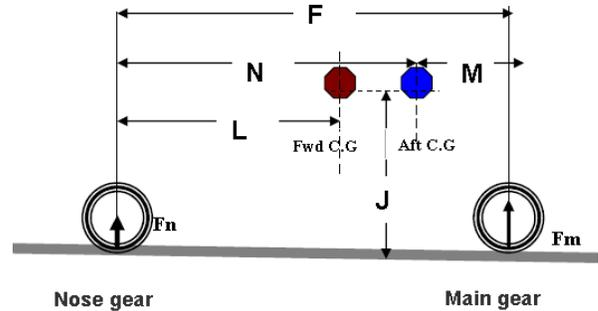
Fig.3: Diagram for Nose landing gear load calculation.
