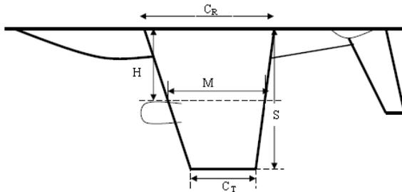
Fig. 2: Half 2-D plan view of UAV for calculation of MAC.
