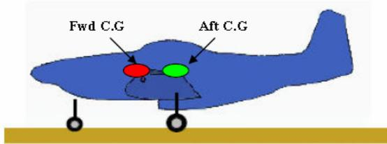
Fig. 1: Aerial vehicle with two c.g. positions.
