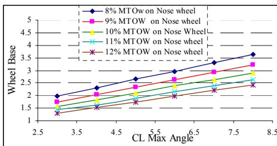
Fig. 7: Nose wheel Vs wheel base at constant angle
