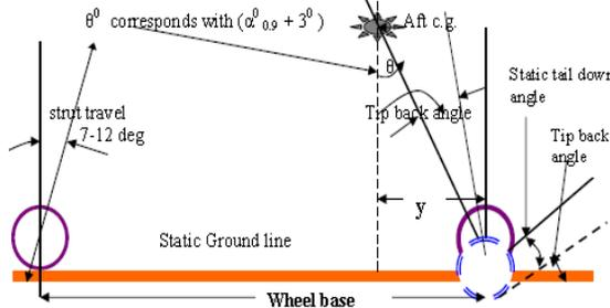
Fig. 6 Tricycle landing gear geometry
