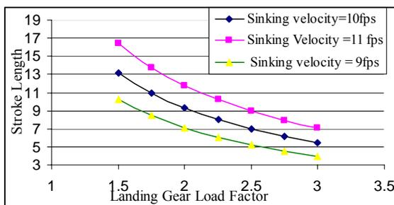
Fig. 9: Vertical wheel travel Vs load factor
