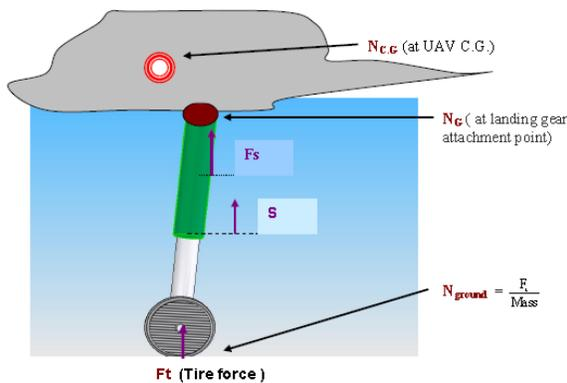
Fig. 4 Shock strut dynamics
