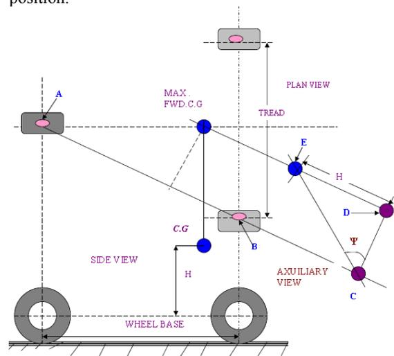
Fig. 5 Wheel track calculation based on turn over angle
