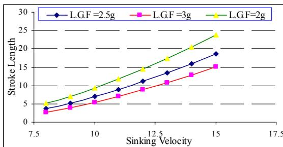
Fig. 8: Sink speed Vs vertical wheel travel
