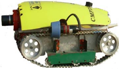
Fig. 4: The Sub-terranean Robot (SR-1) with rigid suspension. This was developed for rescue operation in flooded coal mine galleries.
