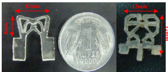
Fig. 8: PDMS grippers fabricated by Vacuum Casting.
