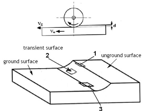
Fig.3: Location of the ground surfaces takes for microscopic study
