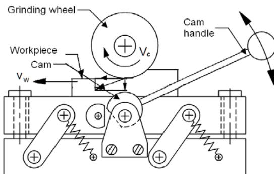
Fig.2: Working principle of quick stop device used in grinding experiment
