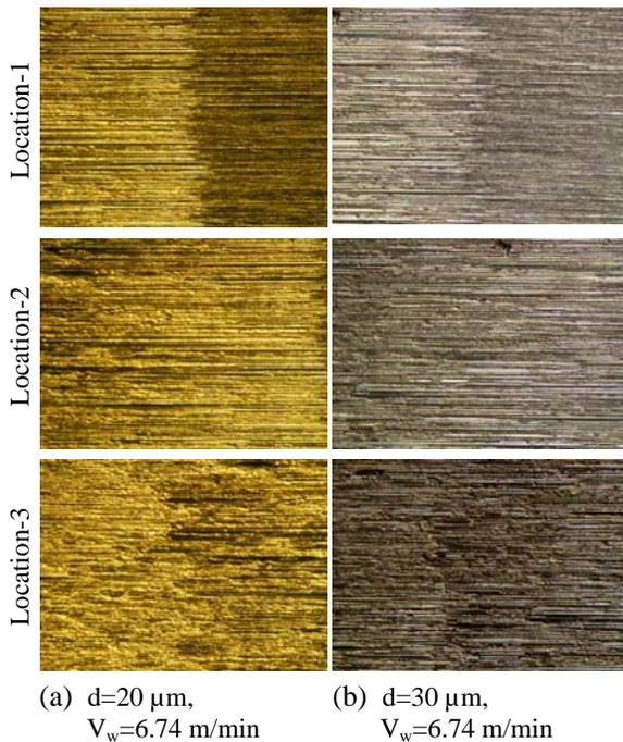
Fig.5: Micro-views of different zones of after freezing grinding at different infeed and moderate  $V_w$  (a)  $d=20 \mu\text{m}$ ,  $V_w=6.74 \text{ m/min}$ , and (b)  $d=30 \mu\text{m}$ ,  $V_w=6.74 \text{ m/min}$
