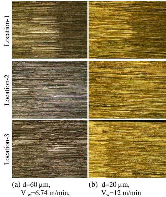
Fig.6: Micro-views of different zones of after freezing grinding at (a)  $d=60 \mu\text{m}$ ,  $V_w=6.74 \text{ m/min}$  and (b)  $d=20 \mu\text{m}$ ,  $V_w=12 \text{ m/min}$
