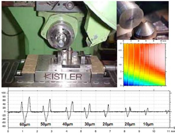
Fig.4: Pattern and sectional profile of the groove formed by the grit in orientation 3.
