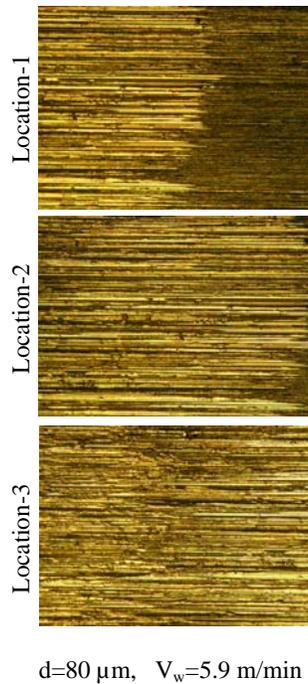
Fig.6: Micro-views of different zones of after freezing grinding at large feed and low  $V_w$  ( $d=80 \mu\text{m}$ ,  $V_w=5.9 \text{ m/min}$ )
