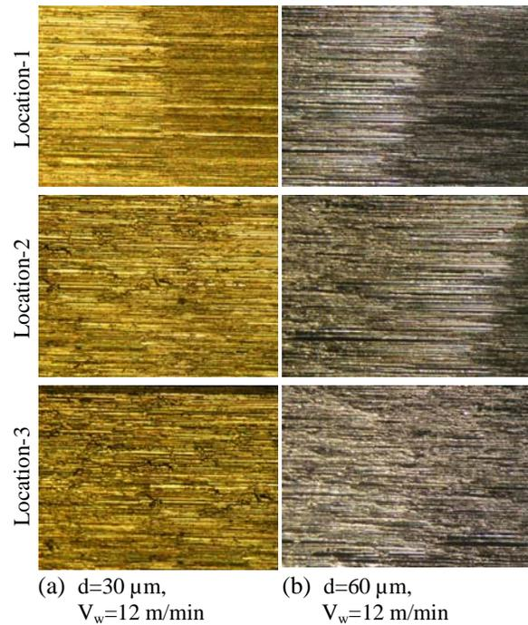
Fig.7: Micro-views of different zones of after freezing grinding at (a)  $d=30 \mu\text{m}$ ,  $V_w=12 \text{ m/min}$  and (b)  $d=60 \mu\text{m}$ ,  $V_w=12 \text{ m/min}$
