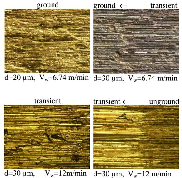
Fig.9: Detail micro-views of the surfaces after freezing grinding at different infeeds and work feeds.
