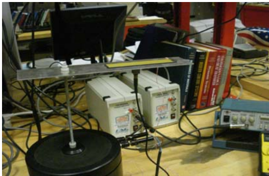
Figure 5: Experimental setup of aluminum beam with piezoelectric actuator for control
