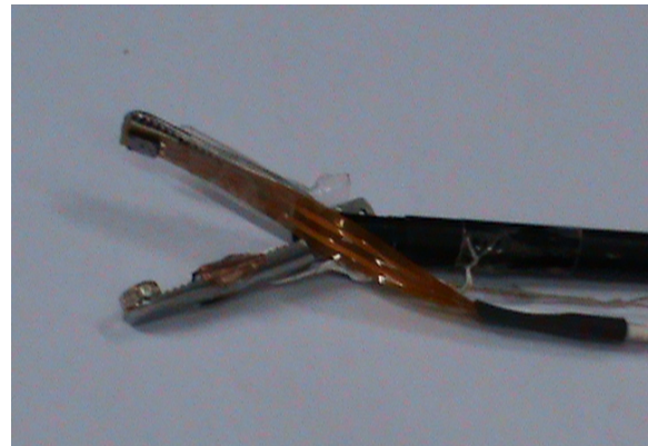
Fig. 14: A laparoscopic gripper with temperature and a small force sensor (3 mm × 3 mm) on its either jaw. The button like object on the lower jaw prevents the damage on the force sensor.
