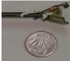
Fig. 12: A laparoscopic gripping tool with force and temperature sensors on its jaws.
