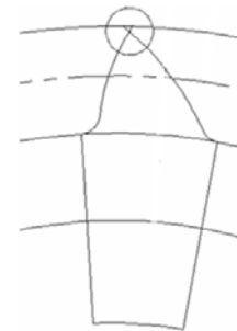
Fig. 13: Gear tooth profile for 20 o /45 o pressure angle
